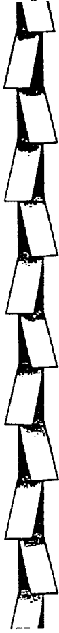
EVERY TOOTH SET (ETS) For cutting soft materials such as non ferrous metals, plastics and wood.
