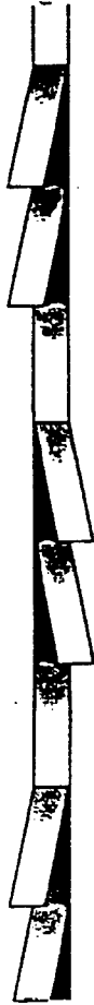
GROUP SET (GS) Is used by smaller tooth pitches on blades for horizontal bandsaw machines. Recommended for cutting exceptionally small dimensions.
