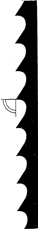
CONVENTIONAL TOOTH (S) rake angle 0^\circ Universal application. Used for cutting of cast iron, cast steel and rolled material (tooth pitches from 3 - 32 tpi).
